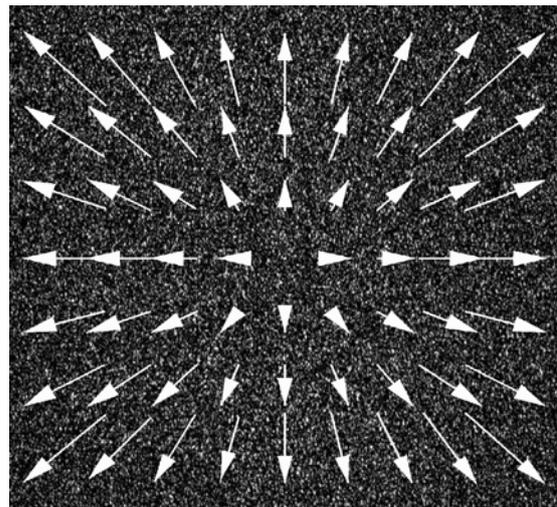
The information about the motion can be retrieved from the speckle dynamics by processing two images of the speckle pattern acquired with a small time lag. Both images are divided into small interrogation areas and cross-correlation functions of such a pair of interrogation areas provides the local displacement of the speckles – see figure. In order to do real-time processing of the expansion/contraction of the speckle pattern spatial-filtering velocimetry can be introduced [1].
