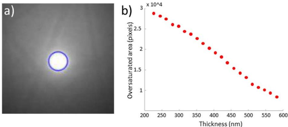
Fig. 2: a) Measurement of the oversaturated area in a Kikuchi diffraction pattern without background removal; b) Relationship between measured direct beam area and thickness of the sample.
