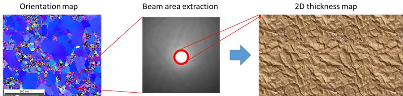
Fig. 3: The overall process of the project: 1) extraction of Kikuchi pattern forming an orientation map; 2) automatic measurement of the diameter of the oversaturated area; 3) Conversion to a relative thickness value and plot of a 2D thickness variation map of the scanned area.
