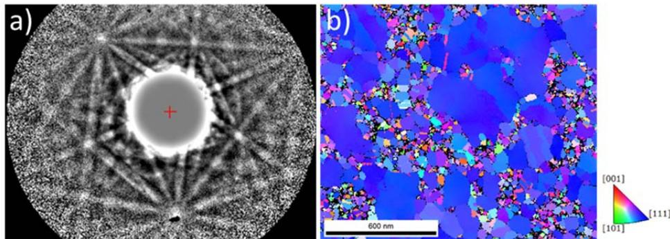
Fig. 1: a) Kikuchi diffraction pattern with background removed, obtained from an Au film; b) Orientation map of a gold film, showing the different crystal orientation of the grains in the film.
