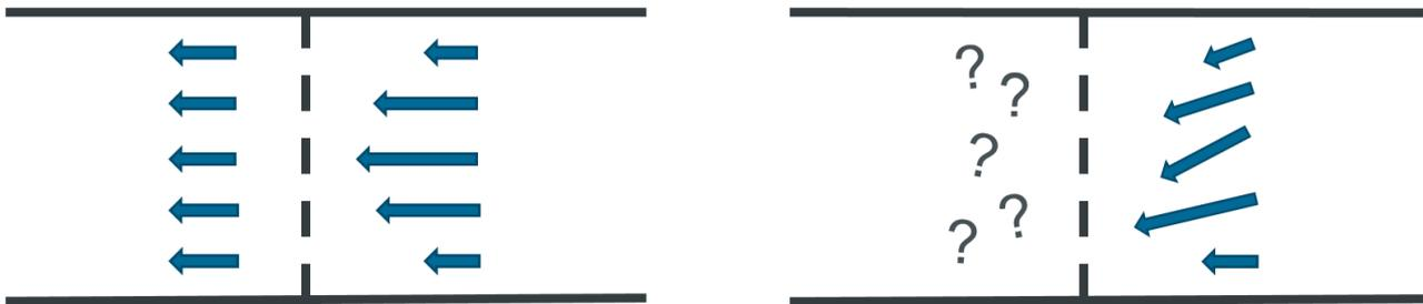
Figure 2: To the left: Perforated plate with flow normal to the plate. To the right: Perforated plate with non-normal flow. This means that the coefficients are unknown, hence the flow downstream is unknown.
