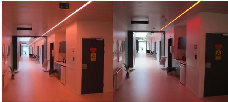
*Middelfart Hospital: Example of integrated lighting design for controlling the level and color temperature of artificial lighting to compliment the natural daylight levels to benefit the health of occupants.*
