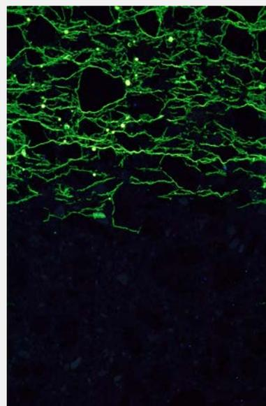
Photo: ASR induced crack extent and propagation in slabs. The ASR induced cracks are visualized as bright green colour.
