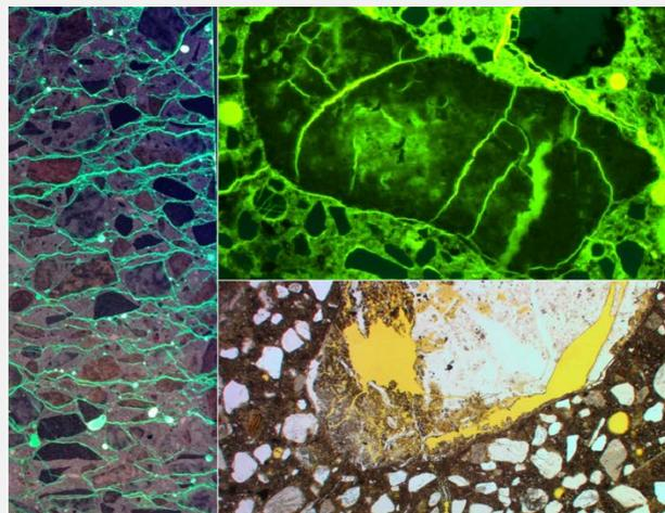
Photo: ASR damaged concrete sample impregnated with fluorescent epoxy and subjected to UV lighting.
