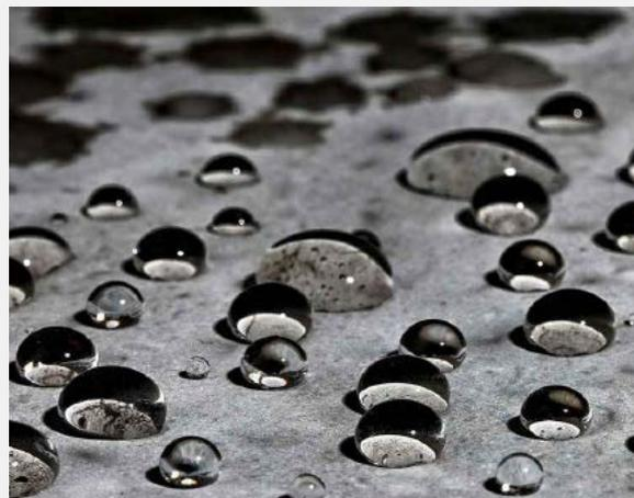
Photo: Water drops on a coated concrete surface.
