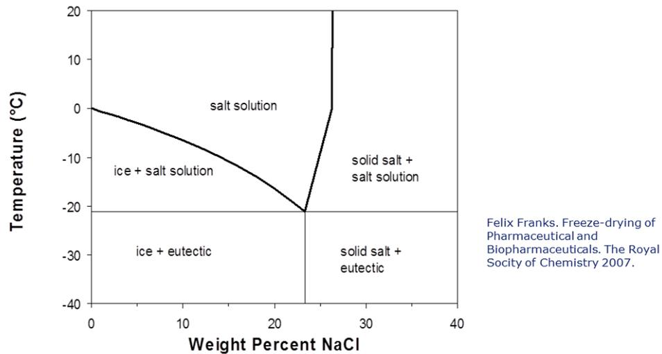
**Figure 4. Freezing behaviour: temperature composition phase diagram for sodium chloride and water.**
