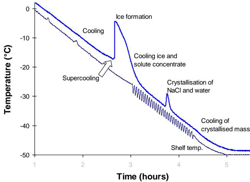
**Figure 5. Product temperature against time during freezing of 5% NaCl (crystalline solute).**
