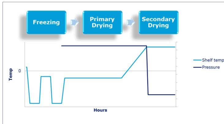
**Figure 3. Freeze drying process including freezing, annealing (thermal treatment), primary drying and secondary drying.**
