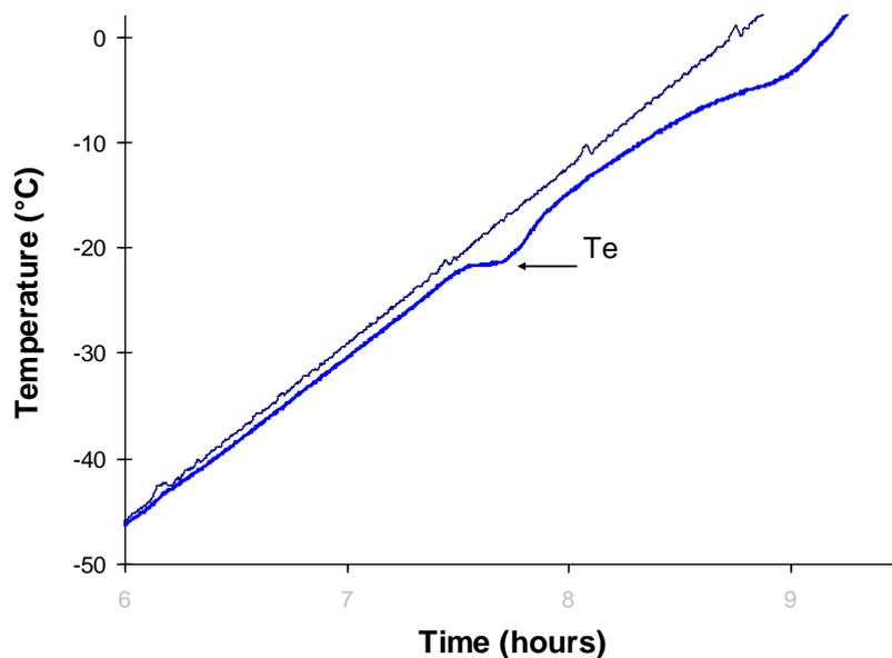
**Figure 6. Product temperature against time during thawing of 5% NaCl.**
