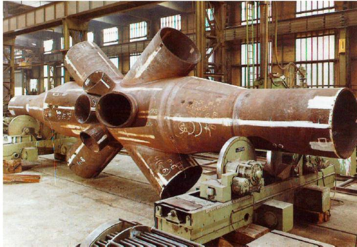
Figure 1 - Complex multiplanar welded joint
